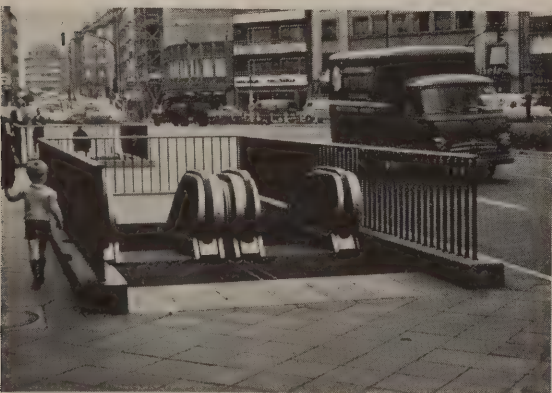
225 An interesting feature of German reconstruction is the use of escalators in the open air. This example from Dusseldorf gives access to a pedestrian subway under a busy road.
